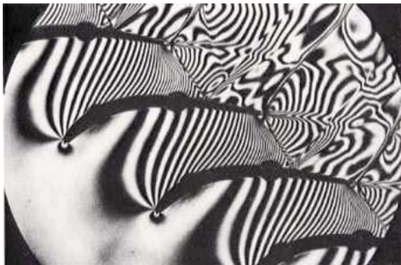
Fig. 17. Flow around driven blade on low-pressure stage in stream turbine (Mach-Zehnder interferometer method).
