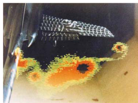
Fig. 22. Total head pattern behind horizontal tail (pressure sensors and light-emitting diodes combination method).
