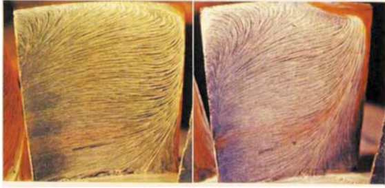
Fig. 11. Oil film pattern on an impeller surface of an axial flow pump (oil film method).
